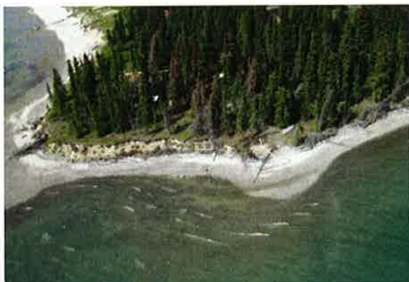
Wave-induced currents along the shoreline transport beach sediment in and out of, or along the shoreline causing sand deposits and erosion.
