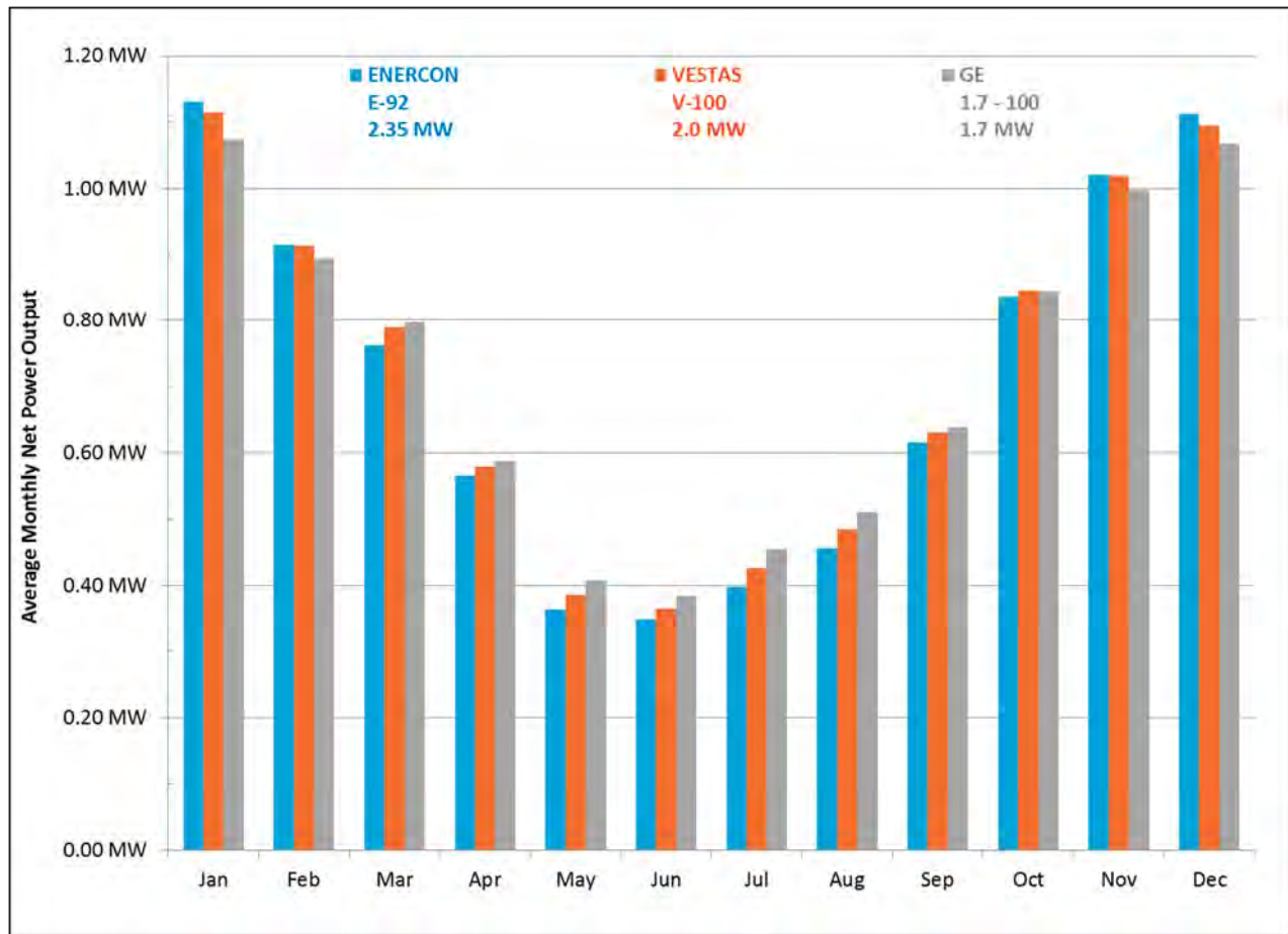
Figure 2 Monthly Generation Profile of a three types of wind turbines at Cyprus Mine Hill
