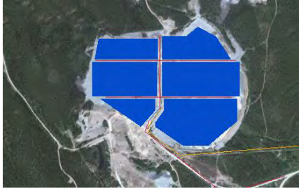
Figure 9.6: 10 MW single axis trackers area requirements at Whitehorse. Only the smallest array options (less than 110 acres – 93 acres shown) will fit.
