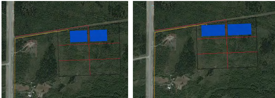
Figure 8.1: 1 MW fixed tilt area requirements at Haines Junction. Left: Smallest (8.5 acres); Right: Largest (13.6 acres)
