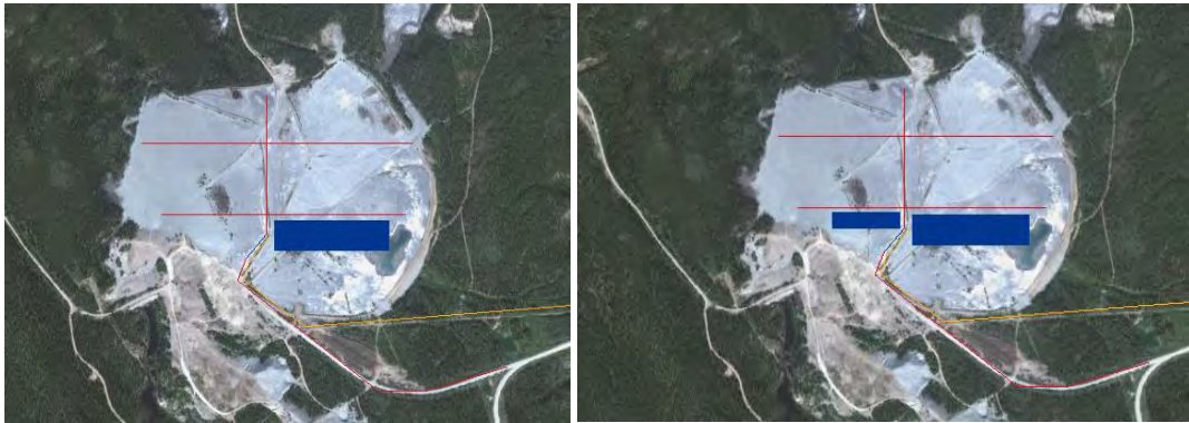
Figure 9.1: 1 MW fixed tilt area requirements at Whitehorse. Left: Smallest (8.5 acres); Right: Largest (13.6 acres)
