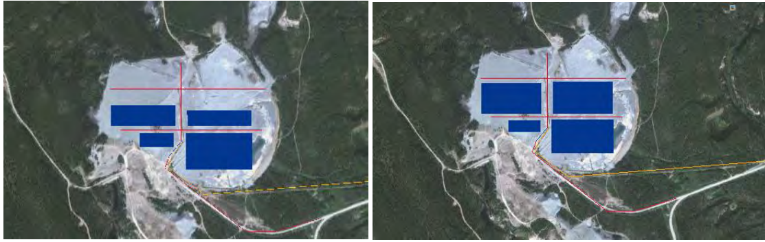
Figure 9.3: 5 MW fixed tilt area requirements at Whitehorse. Left: Smallest (40 acres); Right: Largest (53.6 acres)
