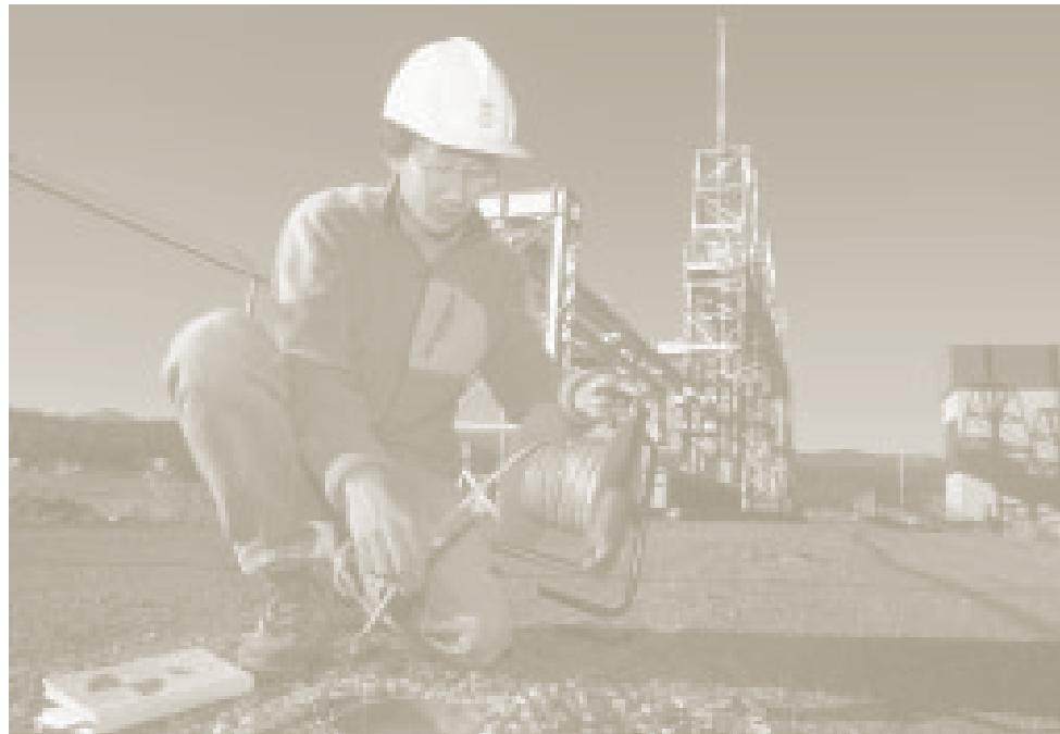
Yukon Energy employee Ron Gee takes readings of water levels in the Whitehorse Dam — Archbould Photography
