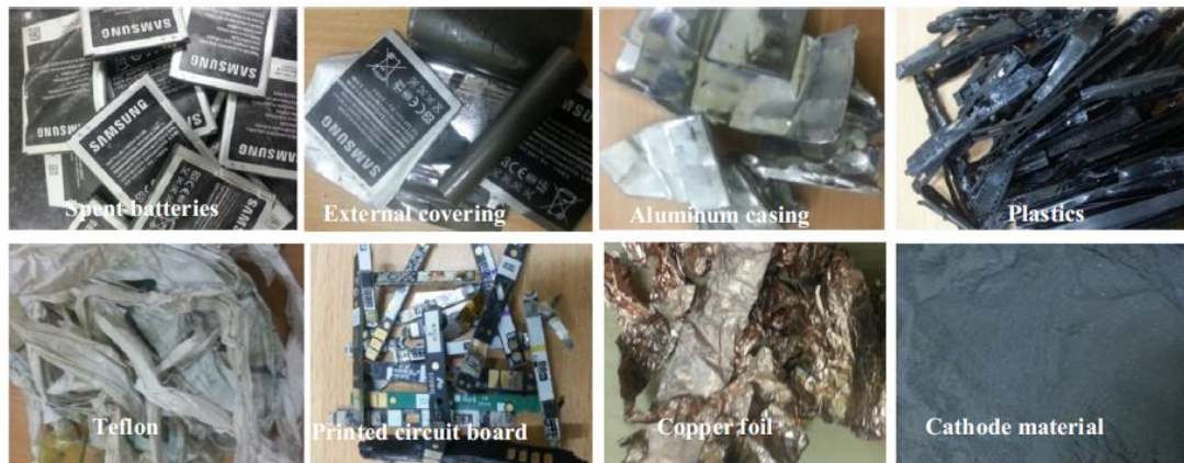
Figure 4-6: Components of Lithium Ion Batteries for recycling, (Barik, Parbaharan, & Kumar, 2016)
