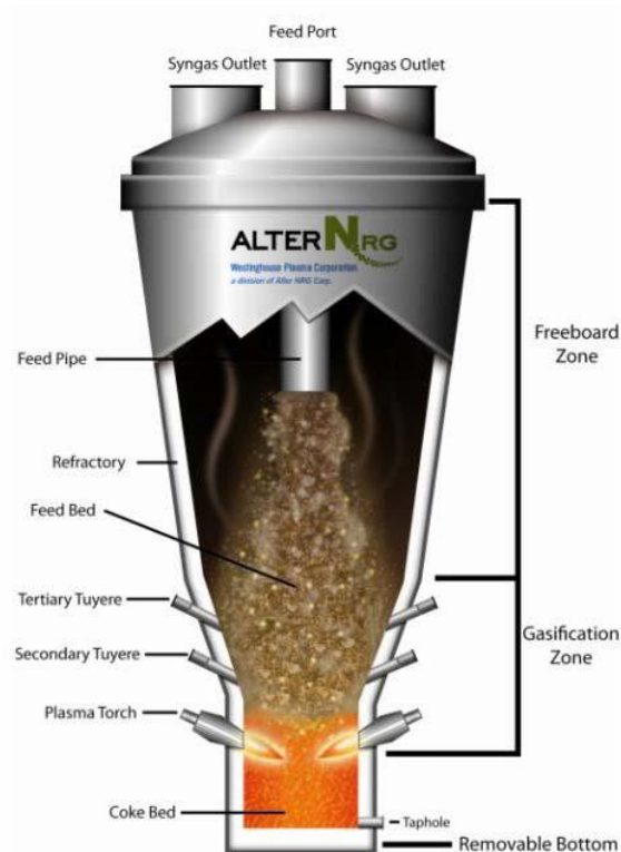
Figure 4-11: Illustration of AlterNRG plasma arc gasifier
