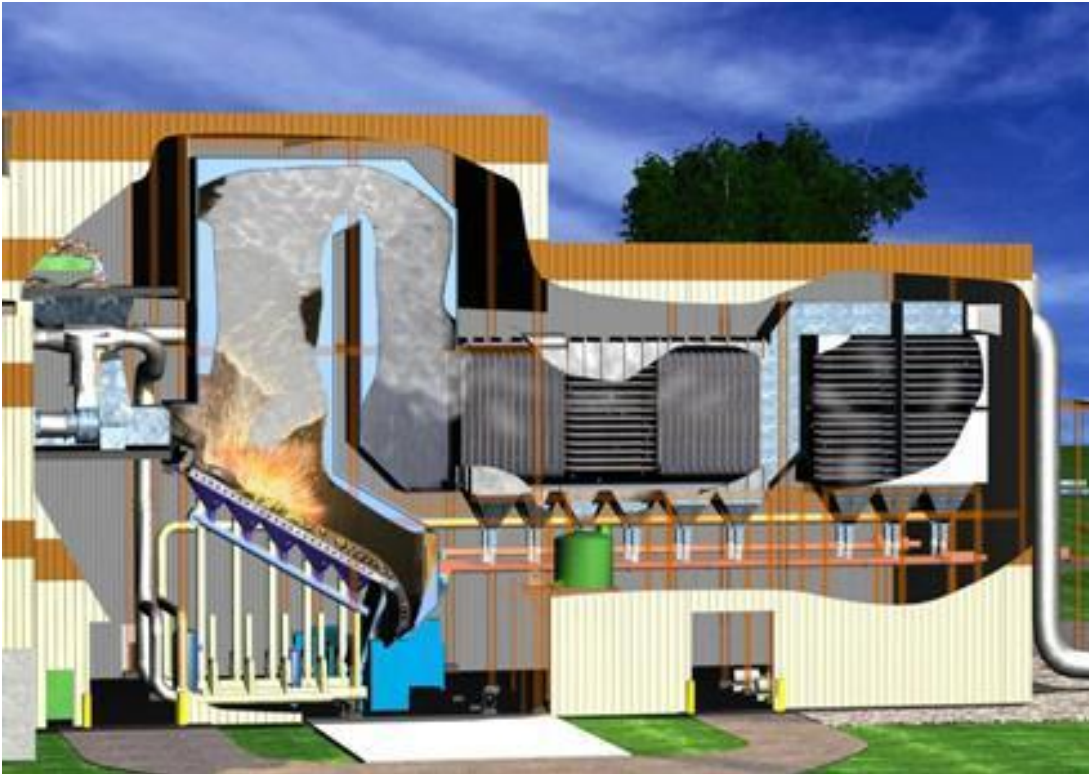
Figure 4-2: Mass burn grate combustion, Novo Energy
