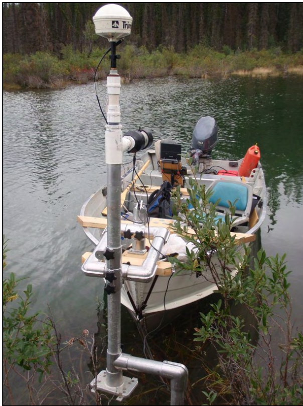
Figure 2. The boat and equipment used to collect the depth and velocity data.
