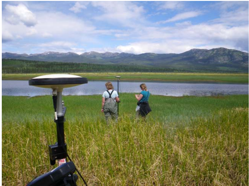
Figure 3. Ecosite unit elevation mapping using Thales DGPS unit at Lewes Marsh (June 6 th , 2010).
