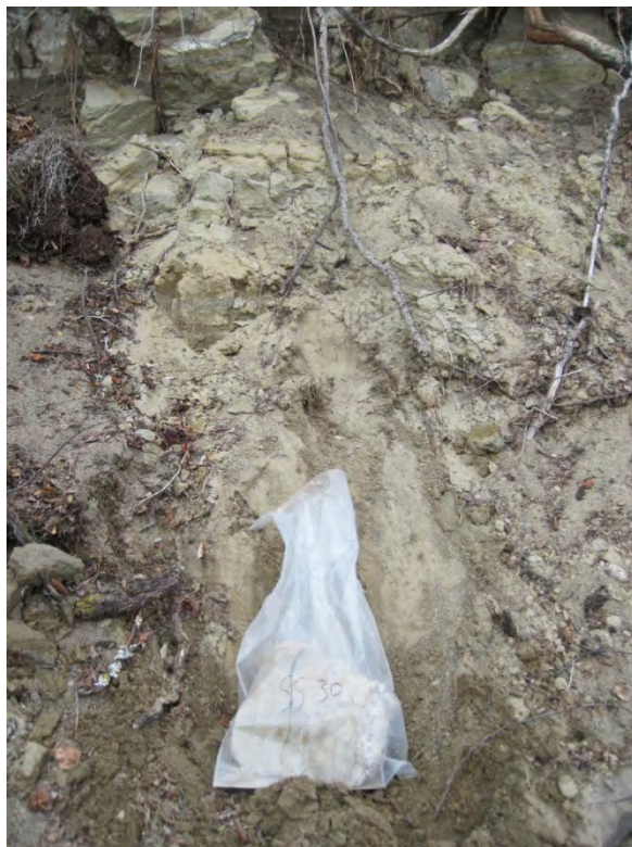
Photograph 7. A sediment sample was collected at the toe of the eroding silt bluff.
