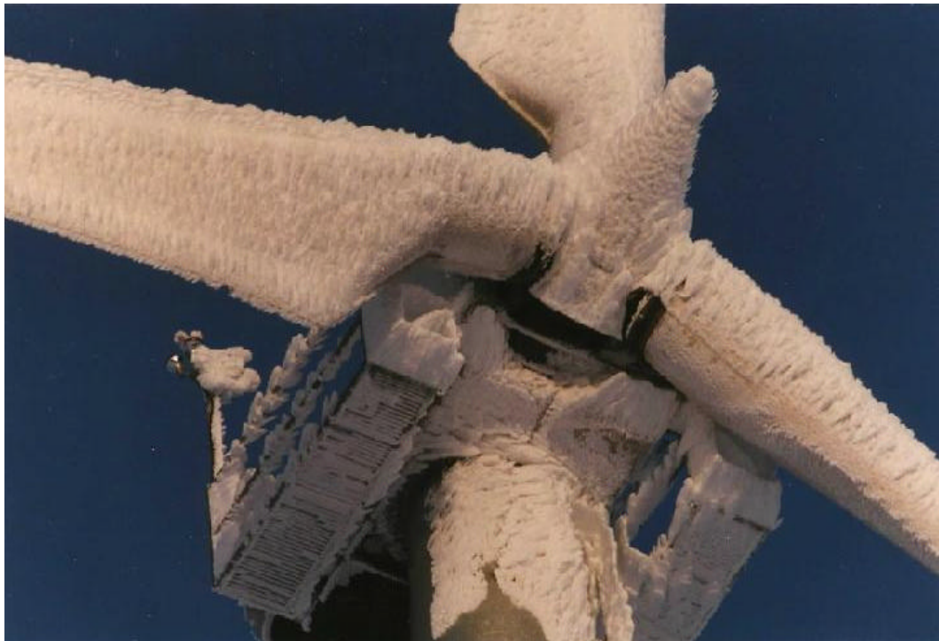
Photograph 4: wedge shaped ice builds up on the blades when running through icing events – leading edge heaters not working
