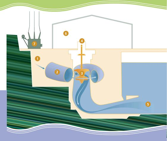
The turbine blades are attached to a big metal rod that has large magnets attached to it. When the blades turn, the rod and magnets spin very fast. The magnets are surrounded by heavy coils of copper wire, and as they spin, electrons in the wire to begin to move, creating electricity.
